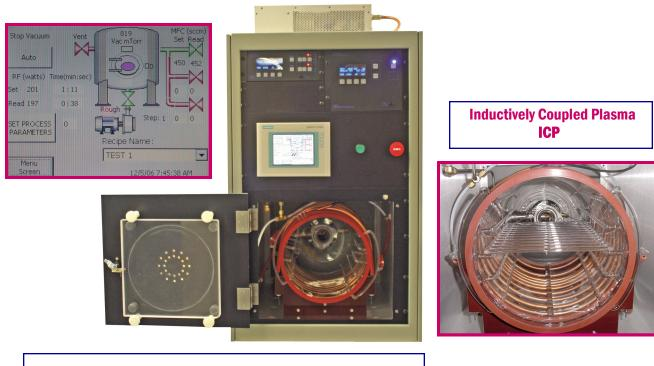
Siemens S7-200 Series "Touch Panel" Control Graphic Operational Display - Pass Word Protected
