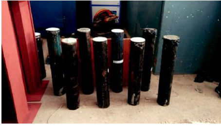
FIGURE 3: CFST columns under self-curing.
