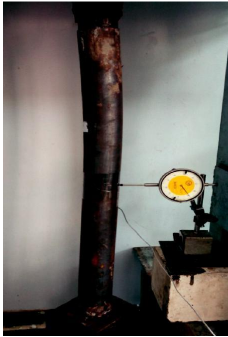
FIGURE 12: Failure of SCFST specimen under axial compression.
