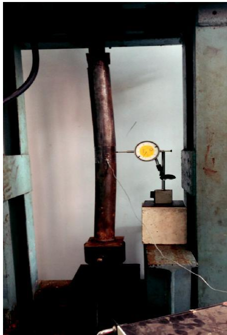
FIGURE 13: Failure of GCFST specimen under axial compression.
