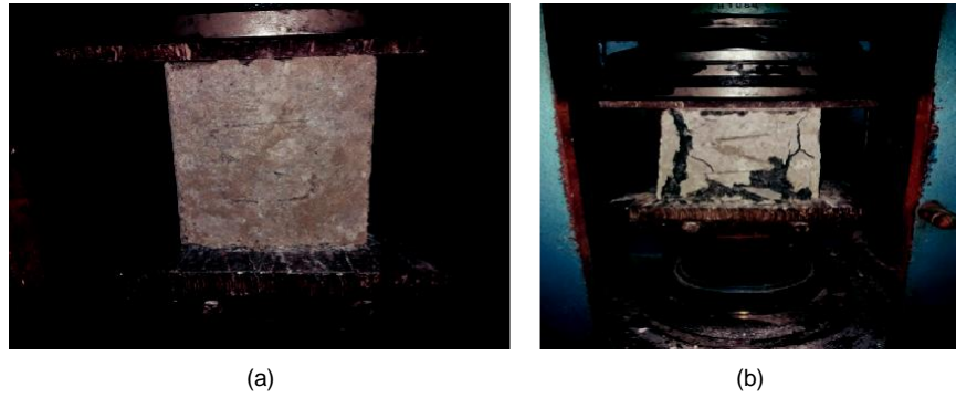
FIGURE 4: Testing of cubes for their compressive strength.
