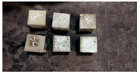
FIGURE 2: Self-curing of concrete cubes.
