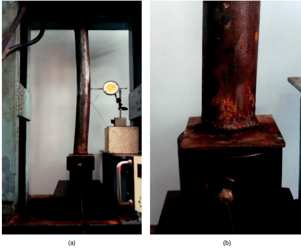
FIGURE 8: Failure of CCFST specimen under axial compression at .
