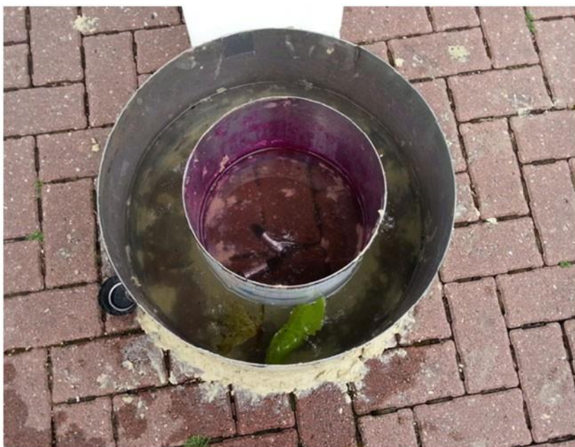
Figure 5. Middle double ring infiltrometer test (two minidivers can be seen in middle ring).
