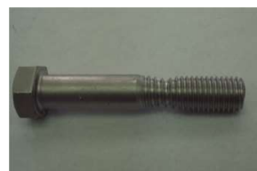
Example of a Ductile Overload
