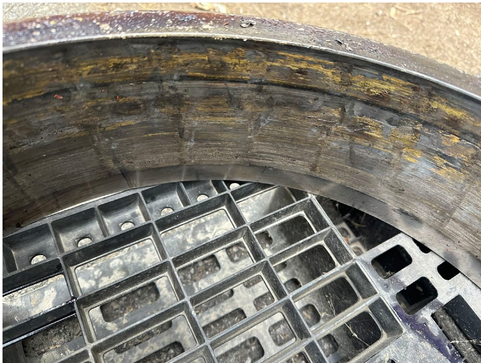
Photo 16 - NDE BRG Raceway w/ Bronze Cage Adhesion
