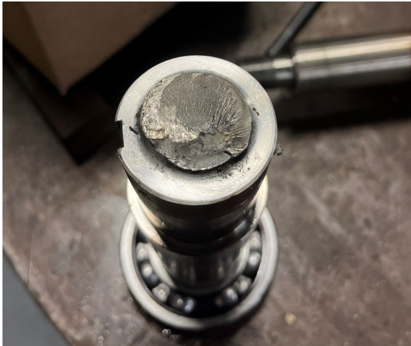
Photo 1 - Pump Shaft Rotational Bending Fatigue Fracture
