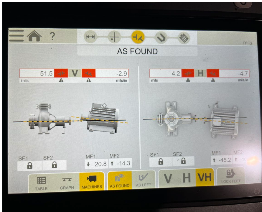
Photo 9 - Misalignment After Pump Piping Disconnected
