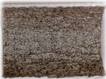
Pitting (Electrical Phenomena)
