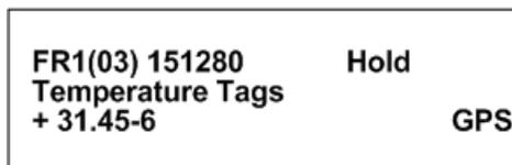
While in **Hold**, the signal strength is not available in the screen, but is recorded to memory with all other available transmitter data. The display will show the converted data, using the entered coefficients for the frequency currently in the display.
