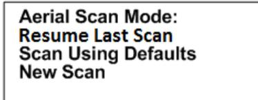
Pressing “**ENTER**” while the cursor is on **Scan Using Defaults**, the Aerial Scan will start up with the values entered in the Aerial Default Menu.
