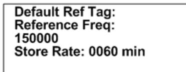
Reference Freq: This is the frequency of a transmitter set up within range of your station used as a check on the system. Since you will not need the same quantity of data you can set up a longer store period to use up less memory. Instead of the strongest signal strength being stored within the storage period, it will be the time of the first valid pulse rate detected.
