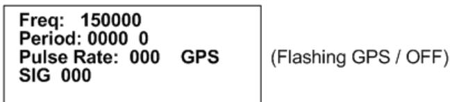
The manual mode does not use pattern matching as the Stationary Mode and Aerial Mode use to detect incoming pulse rates. In the Manual mode screen, the Period and the Pulse Rate are displayed for any two pulses detected. There is a 0-9 single digit counter located after the 4 digit Period. This counter will increment every time a pulse has been detected and will keep incrementing and looping from 0-9 for every duplicate pulse rate. A new pulse rate will clear the count.
