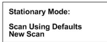
Pressing **“ENTER”** while the cursor is on Scan Using Defaults Scan, the Stationary Scan will start up with the values entered in the Stationary Default Menu.
