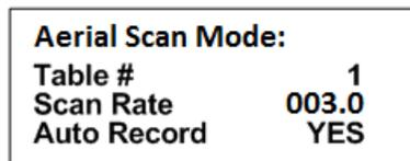
Table #: Selects the frequency table used for scanning. Twelve tables are available. Multiple tables are used to optimize Aerial surveys in multiple locations.
