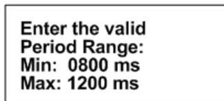
The number entered here should represent the range of pulse rates you are using in your study. The available period range allowed to be entered is between 400ms to 6000ms. The periods measured from signals that are outside the entered range will be thrown out.
