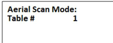
Table #: Typing a new table number and pressing %**ENTER**+ will resume the last scan using just the frequencies from that specific table. Just pressing %**ENTER**+ without typing in a new table number will resume the last scan with all the tables last used. Twelve tables are available.
