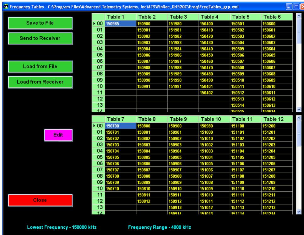
The screens will be the same for viewing a frequency table or editing a frequency table. In the **View Frequency Tables** mode, no parameters can be modified.
