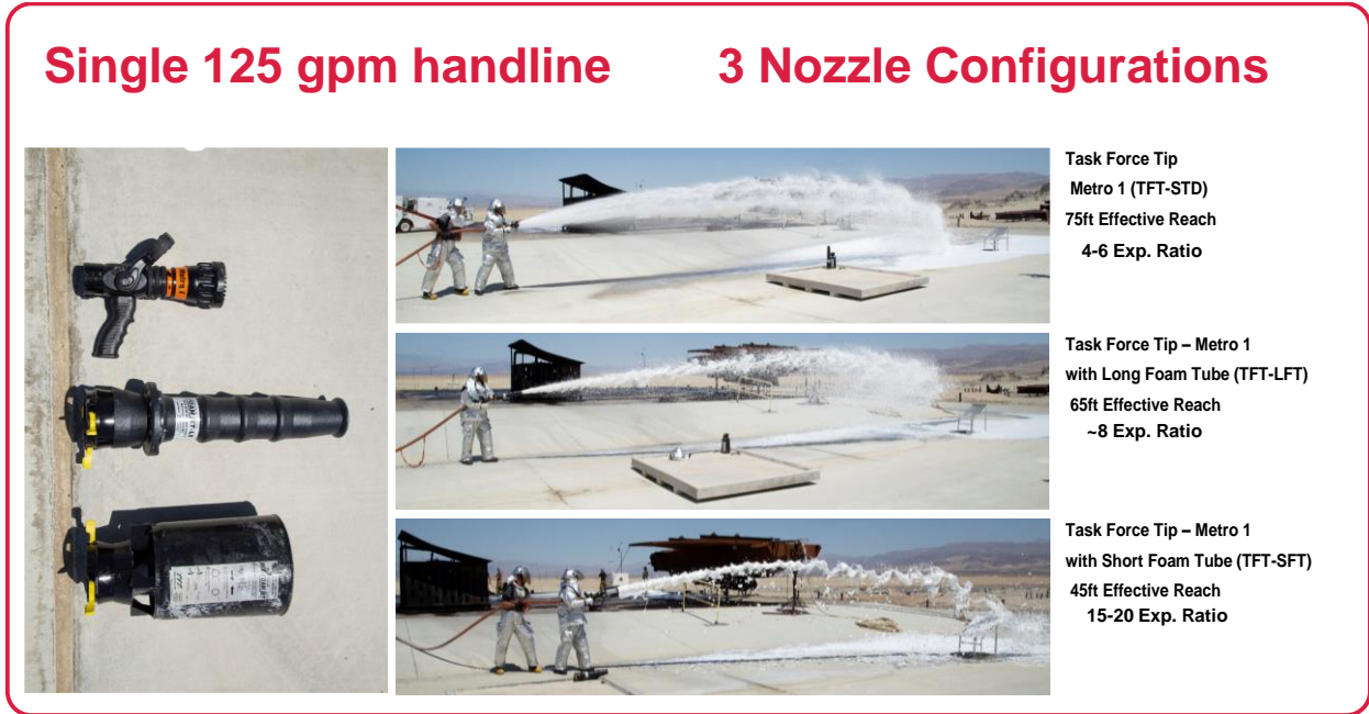
Figure F.4.0-1 Hose Line Nozzle Configurations
