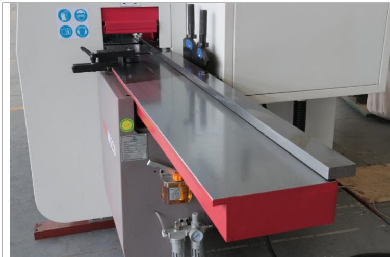
Hard chrome mirror effect feeding table not only anti-rust, but also for a smooth feeding
