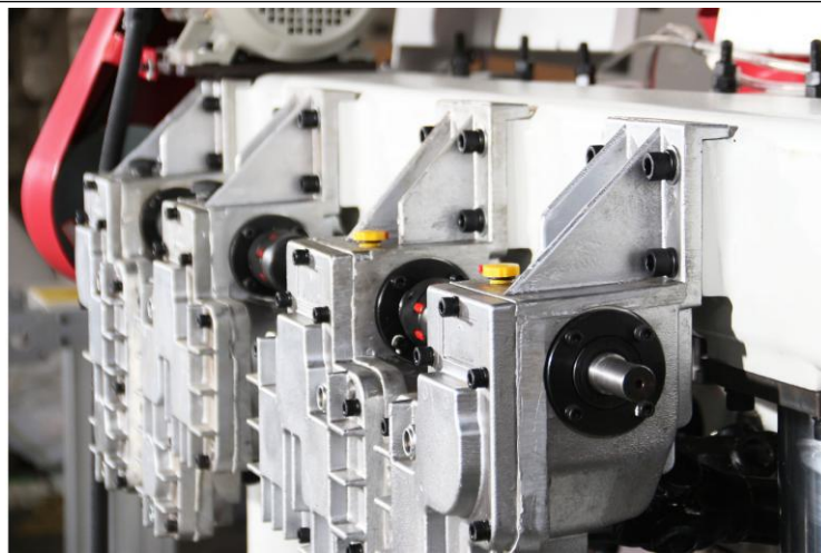
Professional gear synchronic system makes feeding roller running at same speed to give a smooth feeding and further ensure the precise moulding work
