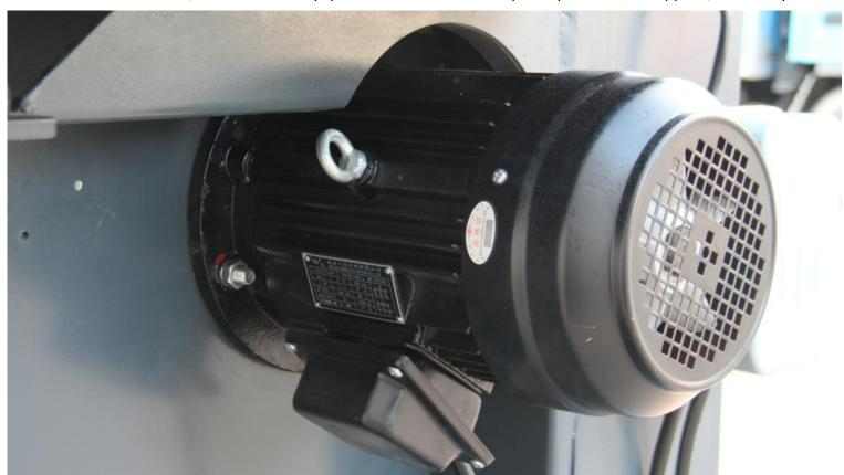
The 4kW motor CE certified model gives very powerful running and got electrical breaking function
