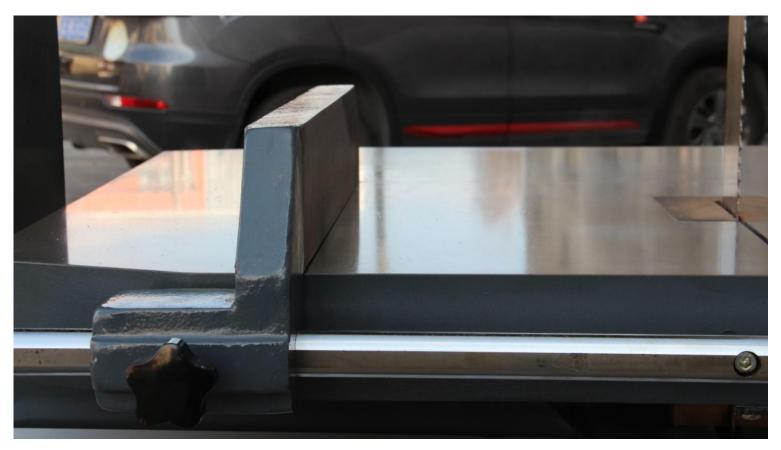
Solid cast iron mirror like grinding for smooth feeding, solid robust rip fence for life long precision.
