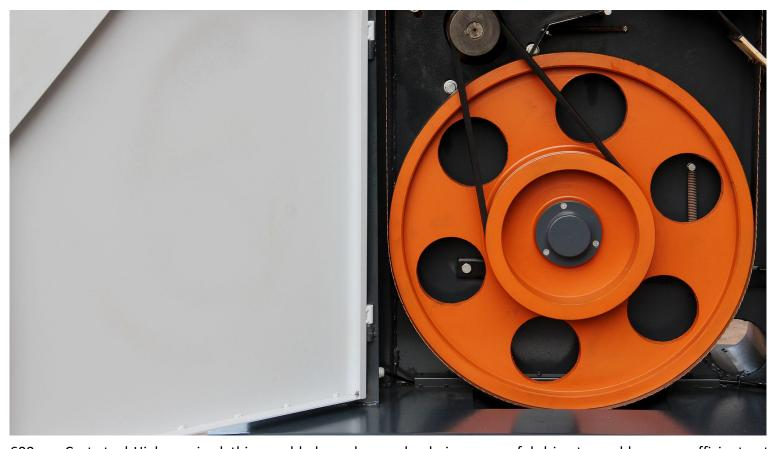
600mm Cast steel High precise lathing and balanced saw wheel gives powerful drive to enable a very efficient cut and perfect cutting surface.
