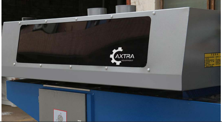
100mm dust collection mouth 1 on bottom 2 pcs on top of big cover gives a very effective dust collection, makes working condition away from dust
