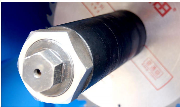
Industrial 60mm diameter spindle is a reflection of a industrial heavy duty rip saw
