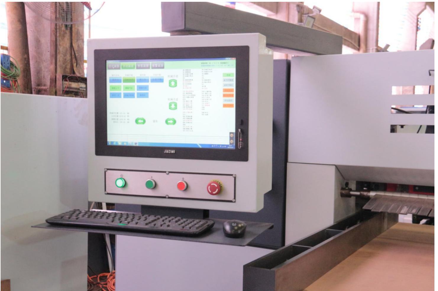
Big control interface with windows program, both touching control and key board mouse control.
