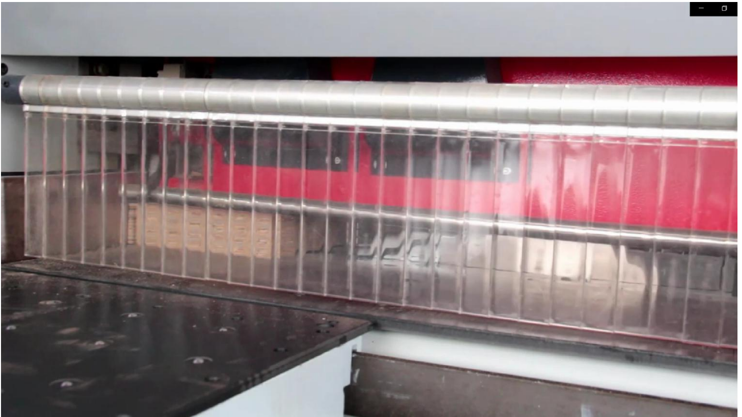
Absolutely safe: harden curtain cover, no chance for user to approach blade
