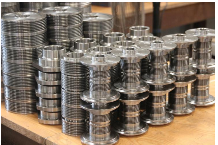
Fine processing of saw spindle to avoid any error of cutting
