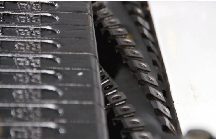
Axtra Silent power black harden spiral cutter makes planing very easy even for big amount planing
