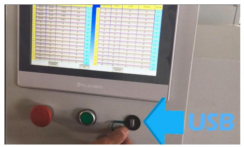
USE control panel directly on machine to set cutting program or use USB to download excel format documents to machine, very flexible and easy setting, there are 6 different cutting models available on machine and more can be customized.
