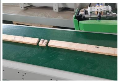
The machine can easy read florescent mark and make a defect cutting according to the mark at speed of 30m/min, the error is less than 1mm
