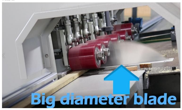
Blade jump is controlled by quick action servo motor with a crank system give a very soft cutting angle rather than direct crash which may cause end break, is the key point for a very clean cutting surface, and even the approaching and leaving angle of blade can be adjust and certainly this mechanical model blade jump system is super stable for life long use.
