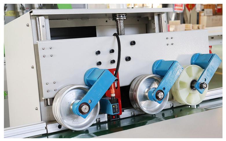
Scanning system also fast reaction is crucial for a precise cutting, it can read the florescent marking and length of material and give the main cutting saw the date, so it is equal to the eyes of machine.
