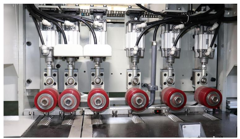
Extremely fast action of pressure top and bottom roller ensure a very fast but same time high accuracy cutting, even the material got slight bending, the multi roller will give a very good holding to prevent jump or position shift of material
