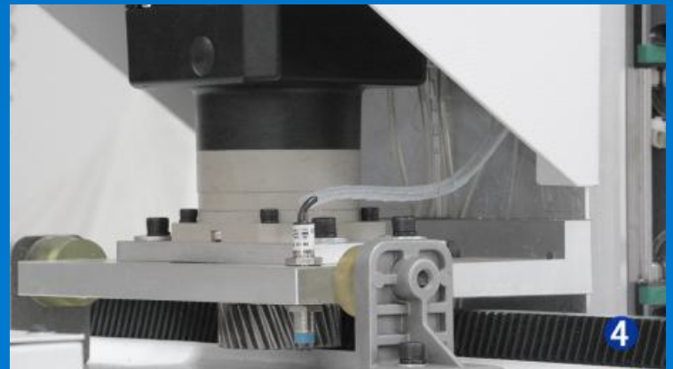
T shape strengthen base for liner rail to endure heavy work
