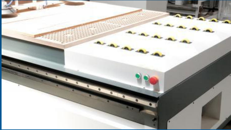
Friendly roller support for easy feeding with remote button control and emergence stop
