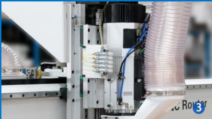
9kW tools change professional high speed spindle the strong heart for a high class machine
