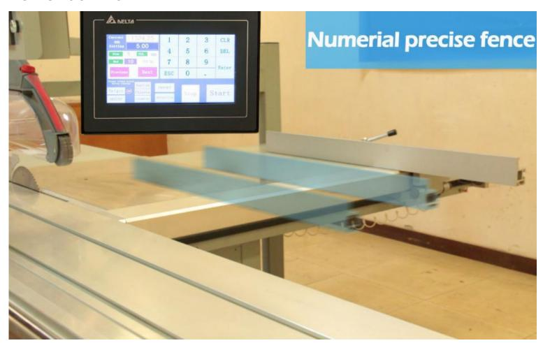
Numerical precise cnc rip fence can be set at a hands reach easy to access super precision avoid tedious double checking of measurement and lock of fence, the fence will move fast at far initial and slower when it near the blade or stop at a safe limit and only can be move by your confirm information this will avoid the collide of blade when you use tilting function.
