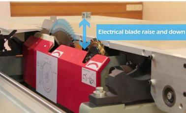
Electrical tilting function can be achieve by a natural Standing control, the motor will stop automatically when the blade reached 45 or 90 degree limit
