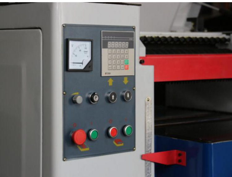
Automatic magnetic scale thickness setting, with speed converting
