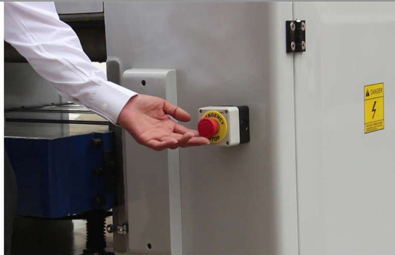
Emergency stop button even at back of machine for ultimate safe
