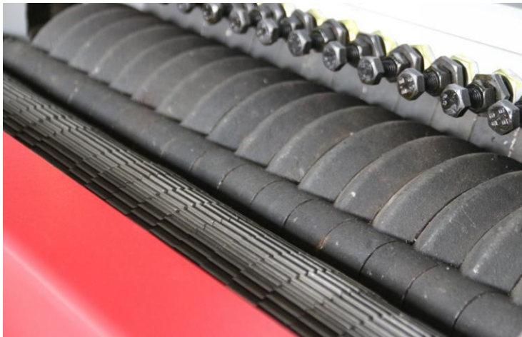
Heavy duty Feeding system with 2 pcs self thickness matching roller and 2 outlet roller and anti jumping system for a super stable feeding
