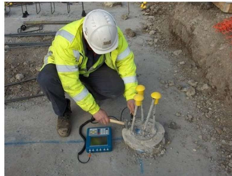
Low strain Integrity test of Pile
