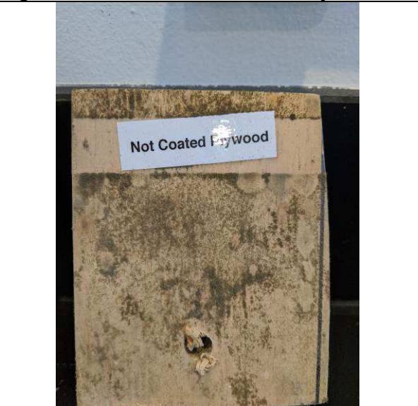
Figure 4. Post-Incubation Control Plywood
