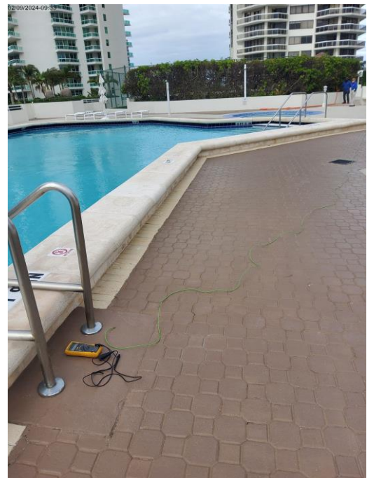
Photo # 100. Item 26.a. Swimming Pool. Pool equipotential bonding: Failed test.
