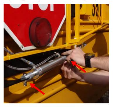
• Wait till end to tighten bolts until end of install once you have confirmed arm is working well.
