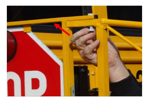
• Tighten nylon nuts to snug with a wrench. Do not overtighten.
