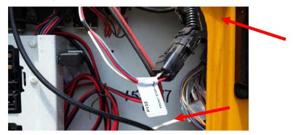
• Cut the blue wire and white wires coming out of the black mollex connector and attach male ends to them. Attach the the splitter to the blue wire. OR keep the molex connector and add male ends to the wires.
