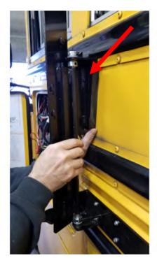
• The top right attachment should be marked, drilled, and a Nutsert used to securely anchor the vertical bracket. Carefully follow Nutsert tool instructions.
