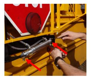
• Secure clevis pin with cotter key at end of install
