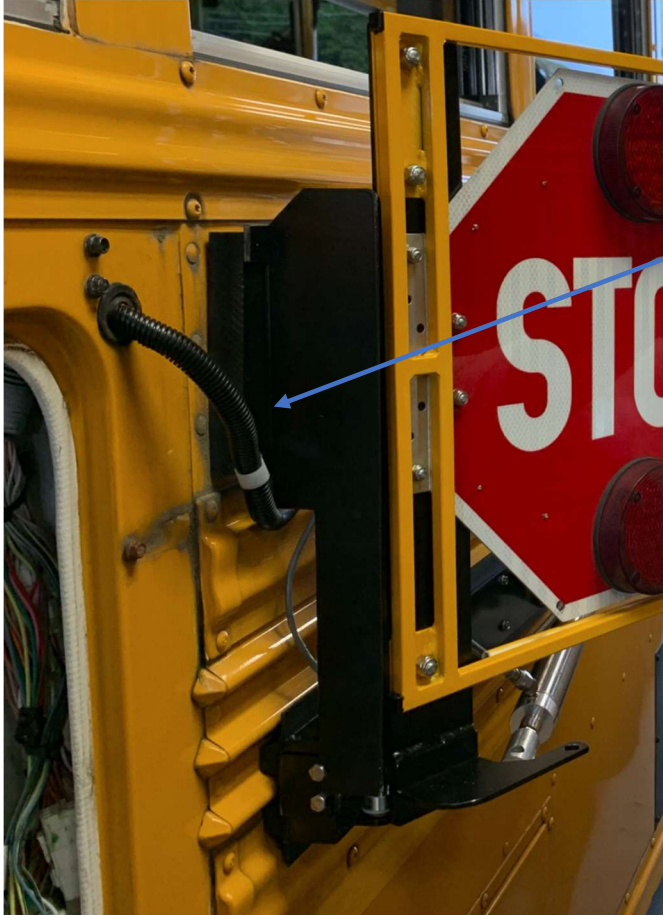
Typical Bluebird Positioning Wire Port in front:
