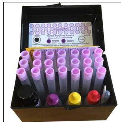
Figure 3. A Nartec MH-21 Marijuana Test Kit, formerly used by MSHP.
