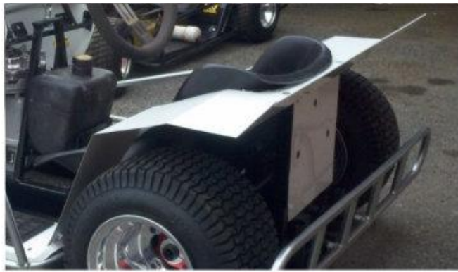
Wrong, has edge.
