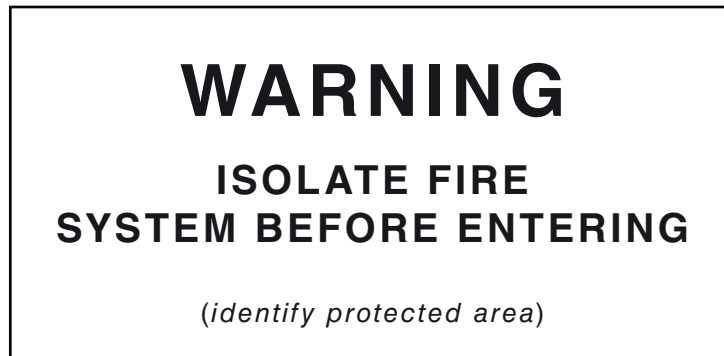
FIGURE 4.4 TYPICAL FIRE SYSTEM ISOLATION WARNING NOTICE
