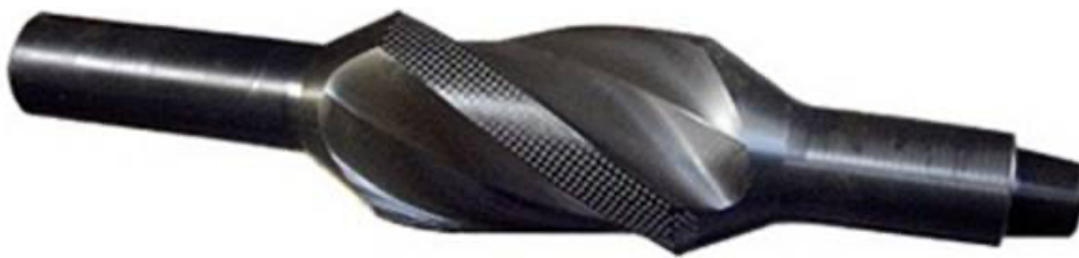
Figure 2: Typical spiral string stabilizer design
