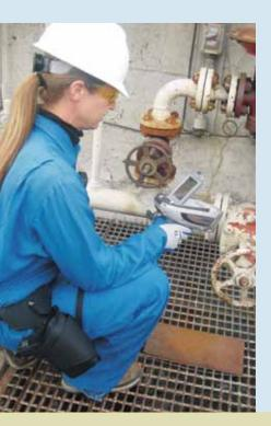
Thermo Scientific GOLDD technology brings true lab-quality performance to handheld XRF analyzers. Delivering up to 10X faster measurement times than conventional technologies, it also provides the highest sensitivity and measurement accuracy, plus the capability of measuring light elements (magnesium, aluminum, silicon, phosphorus, and sulfur) without helium purge or vacuum.
