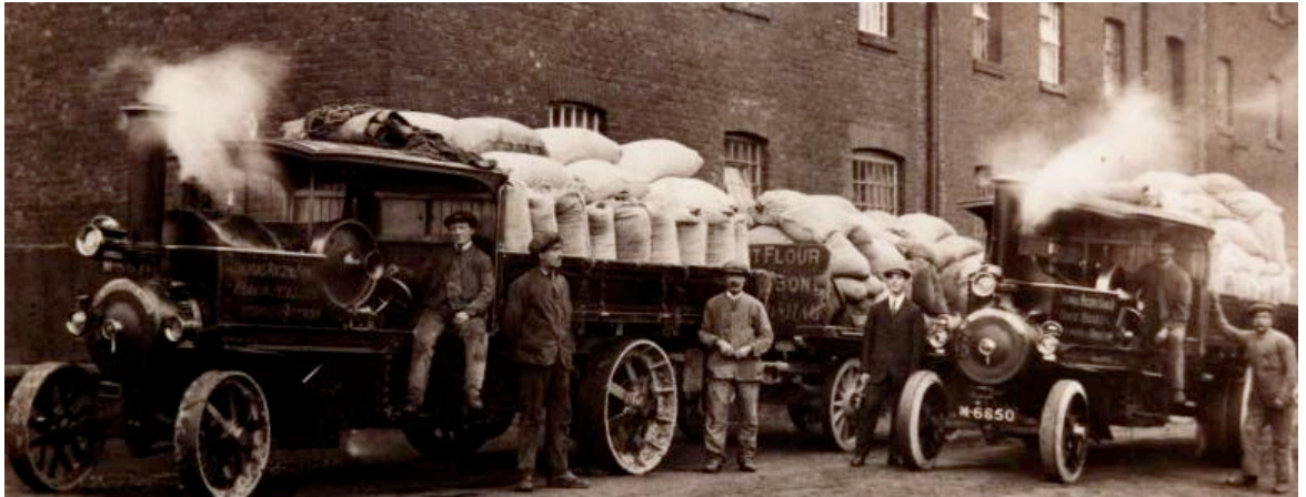
Foden Steam wagons at Thomas Rigby's Sutton Mill, Frodsham - the horses now replaced.
