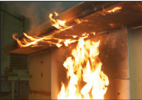
Embers from flames can find their way into your attic through unscreened vents. Photo by Institute for Business and Home Safety Research Center.
