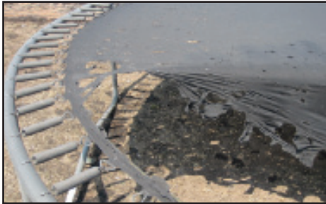
Embers destroyed this trampoline.
