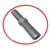
This scaffold fitting connects two scaffold tubes externally. A centre steel divider ensures an equal insertion of each tube. Fitting can be used where tension joints are required particularly useful for long bracing tubes.
