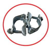
This scaffold fitting connects two scaffold tubes at any angle to provide a ledge brace, front or similar bracing to a scaffold structure. It is a load bearing fitting.
