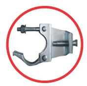
This fitting provides a rotating coupling of a scaffold tube to an "I" beam girder and must be used in pairs with one on each opposite flanges.
