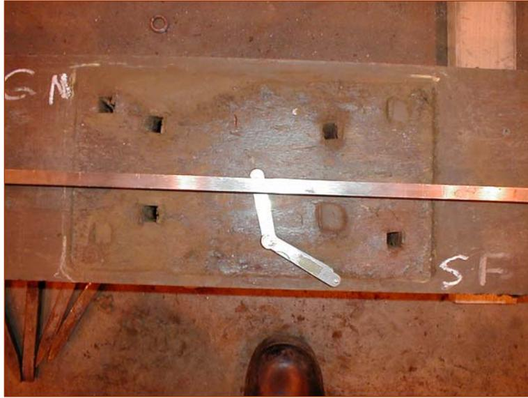
Figure 2. Tie Cutting Measurement Setup
