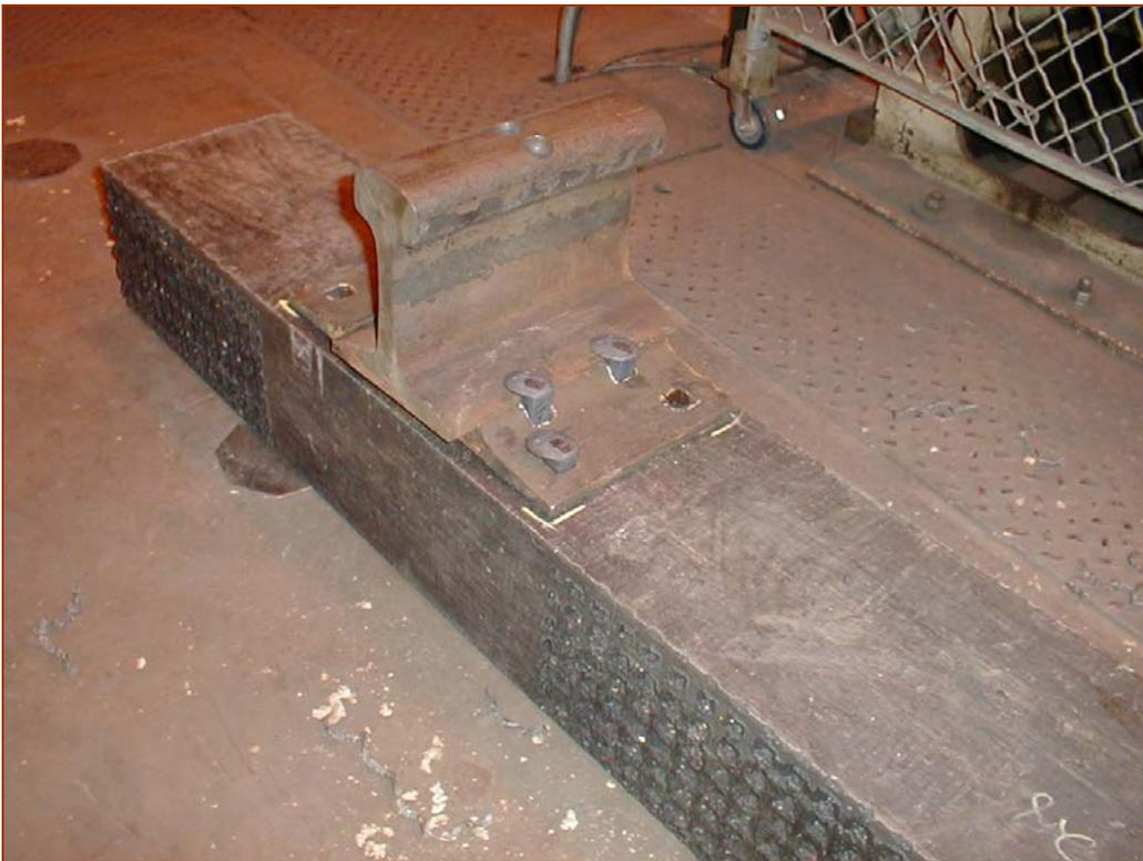
**Figure A-3. Tie Plate and Rail Spiked to Tie**
