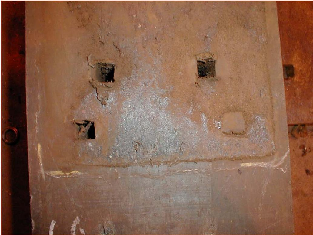
**Figure A-7. Close-up tie Plate Cutting Gage Side**
