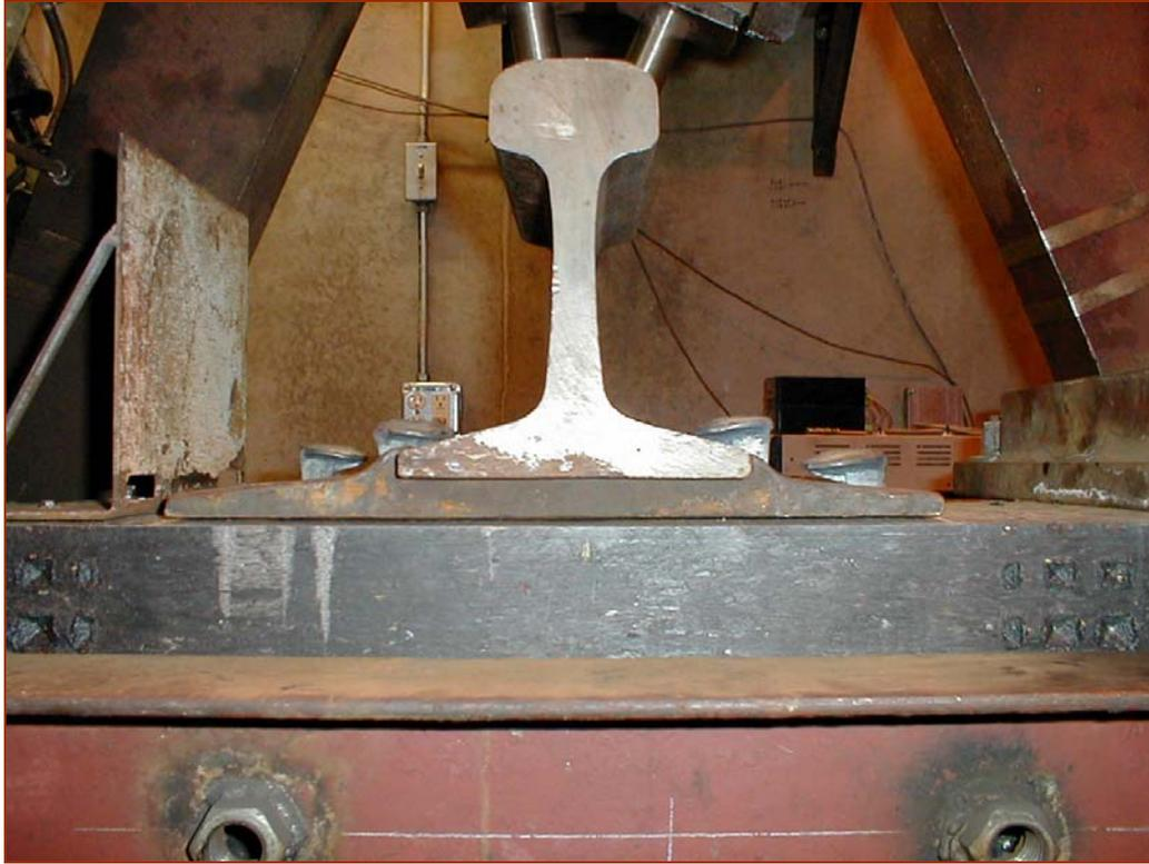
**Figure A-4. Gap between Tie Plate and Tie**
