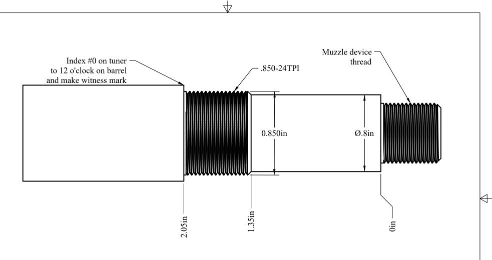
\*\*\* Screws on tuner are tension screws, not set screws. Set them tight enough that tuner can be turned without tools but tight enough that tuner won't turn on it's own. Once best tuner setting is found, you can set them tight enough to act as set screws if desired. Screws have nylon tips, so they won't damage threads unless set extremely tight.
