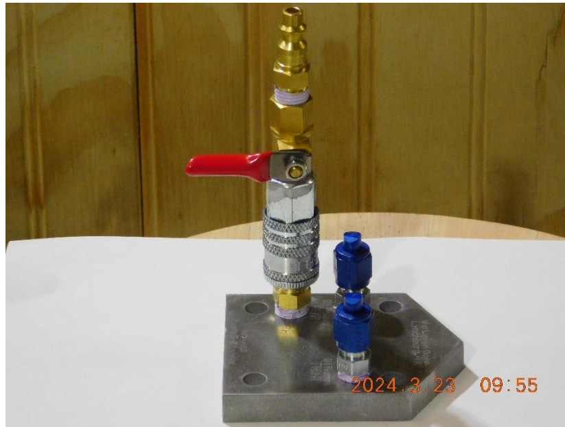
Image 3. MC-483 Test Plate (assembled with quick connect adapter with ¼ turn shut off valve)
