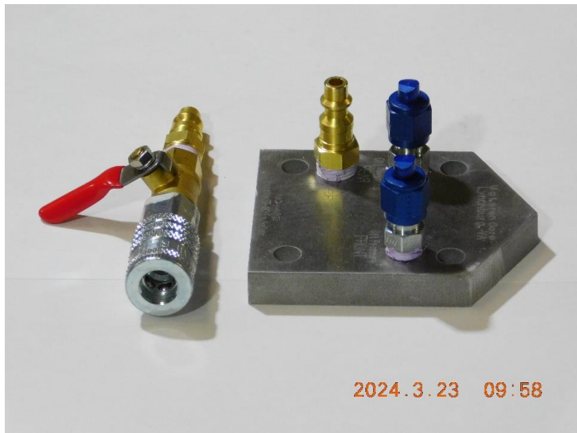
Image 2. MC-483 Test Plate (assembled with quick connect adapter with ¼ turn shut off valve)
