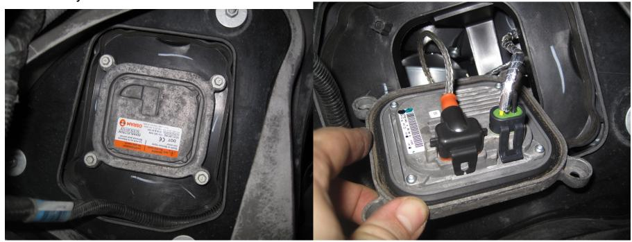
8. Insert the D2S/AMP adapter from the wheel well side of the headlight and fish the AMP connectors through until you feel them in the bottom of the headlight housing and pull it through just enough to make the connections.
