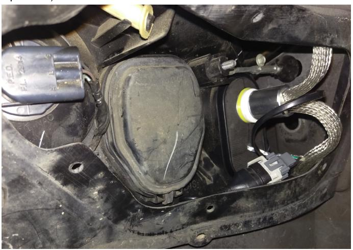
6. Disconnect and Remove the low beam bulb by removing the two T10 screws on the retaining clip. (If you drop these, don't worry, you can scoop them up with your fingers once the bulb is removed) Carefully insert the D2S bulb in the low beam location and secure it with the factory bulb retaining clip.
