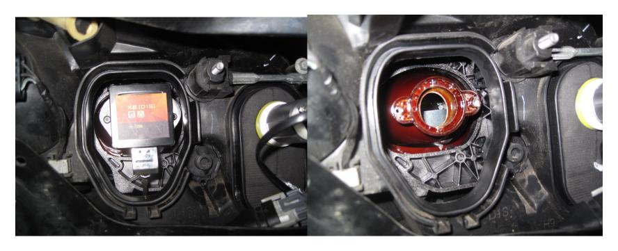
7. Back on the underside, remove the HID ballast from the bottom of the headlight housing by removing the four 7mm screws You'll see 2 connectors. Remove the connector with the green seal. Gently remove the HID ballast and the rest of the harness connected to it. Set this aside.
