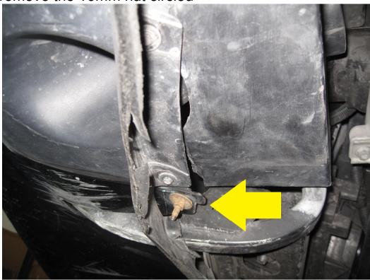
3. Remove the shown panel pins. The access panel and front of wheel well can be removed in a
