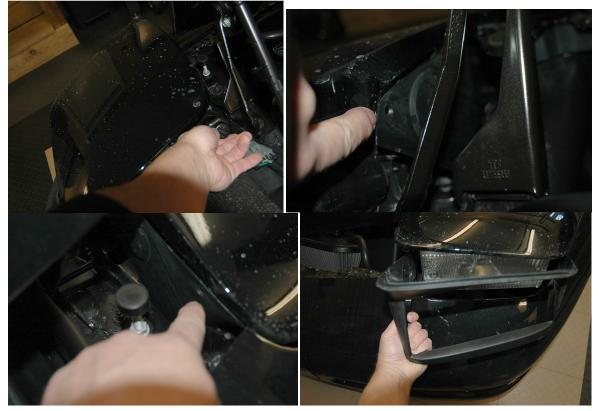
2. Next remove the 4 torx 15 screws that hold the headlight cover in place. 2 are on the back and there's one on each side. Remove these and the headlight cover. Be sure not to lose the plastic or metal sleeve for the bolts.
