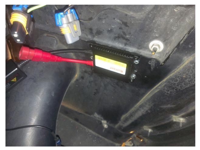
3. Connect the Factory low beam connector directly to the ballast. You will need to plug the ballast the connector in backwards to get correct polarity. When done correctly, the locking clips will be on the opposite side of the locking tab.
