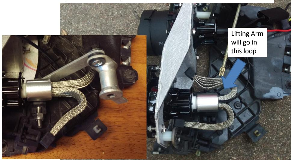
19. Clean off a surface below the headlight bracket and mount the HID ballast. Connect the HID ballast to the low beam factory connector (the one with brown and black wires). Note the +/- signs on the HID ballast connector.
