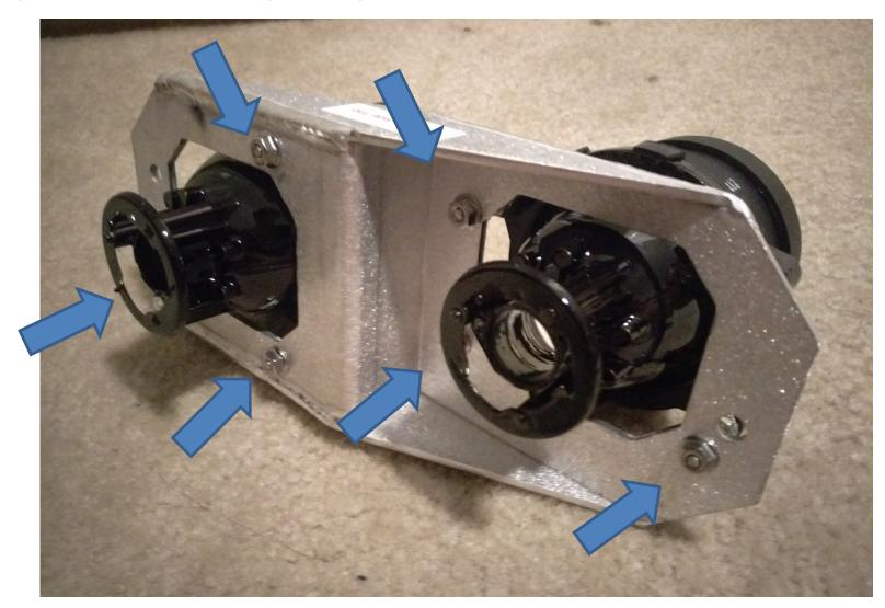
15. Mount the Luminator assembly to the factory headlight assembly using the  $\frac{1}{4}$ " bolts,  $\frac{1}{4}$ " spacers and  $\frac{1}{4}$ " nylon locking nuts as shown.
