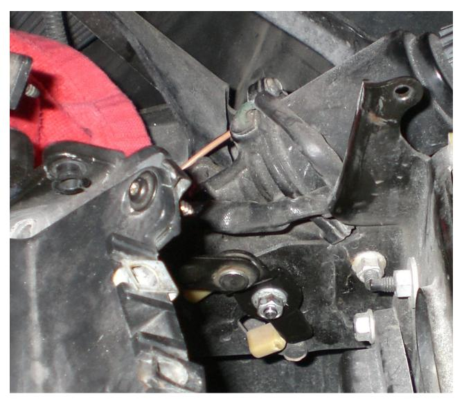
7. Remove the three 10mm mounting screws that hold the headlight reflector assembly to the rest of the headlight assembly.
