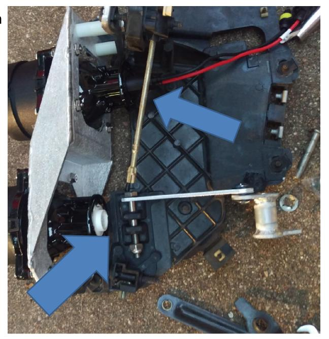
18. Install LED high beam bulbs and twist-lock into the high beam projector. Fold over the heat sink mesh bands so the lifting arm sits inside the looped band. (ref: photos)
