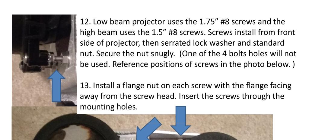
14. Install the second flange nut with the flange facing towards the screw head. Adjust the front and rear flange nuts until the tip of the screw is flush with the backside of the rear flange nut. Tighten the nuts by hand as these may be adjusted later.
