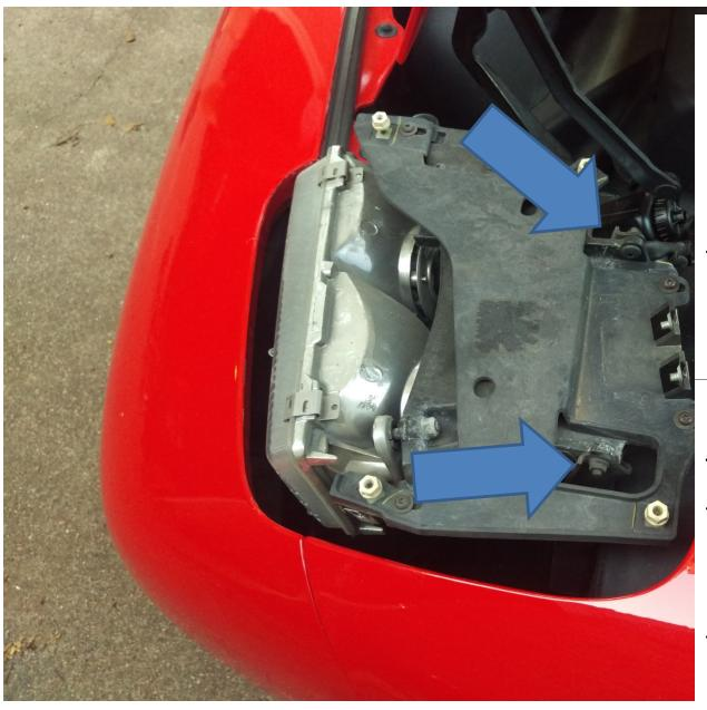
5. Apply WD-40, PB blaster or other penetrating lubricant to the hinge bolts. Allow a few minutes to penetrate.
