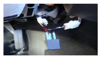
7) Disconnect those plugs and insert your hyperflash harness. Test out your flashers. The car must be started or the lights on. If everything checks out tuck away the harness and reverse the above directions. The flasher will have its own unique click sound. This is normal.
