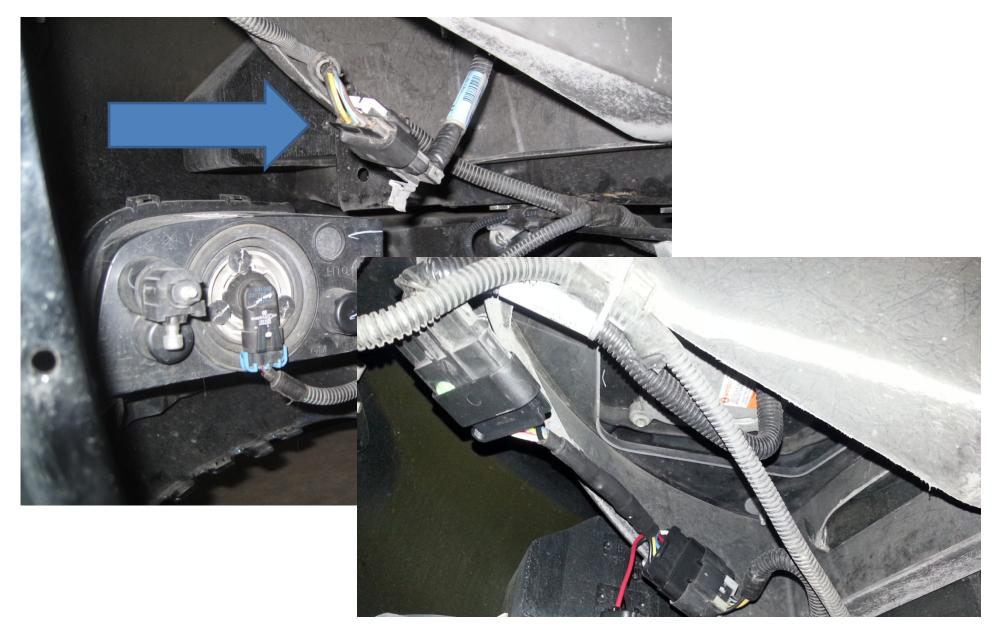
6. Disconnect the fog light bulb and remove the fog light assembly by removing the three 7mm screws on the bottom of the assembly (The fog light removal will allow ease of installation with another opening for your arm)
