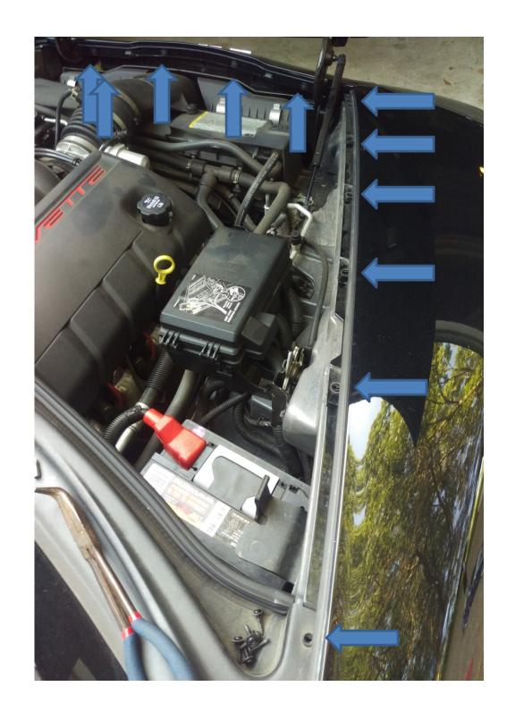
Firmly lift the front bumper to reveal an additional Torx 15 screw on the fender. Remove this screw.
