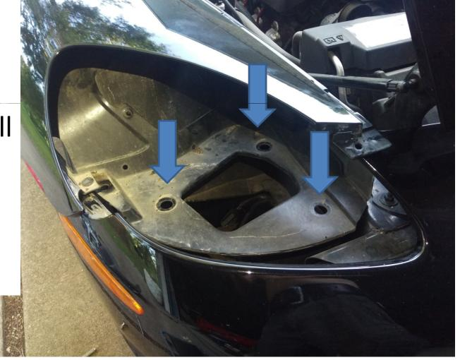
9. Install your new headlights by sliding them in the same way the old ones slid out. Be sure the harness and all it's components drop through the large central cutout. Connect your headlight to the factory connector.
