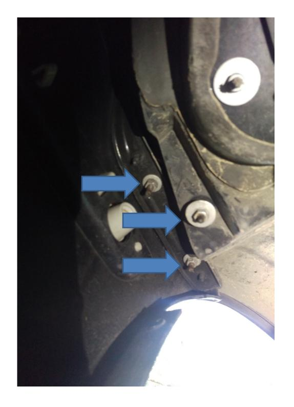
8. Three 10mm nuts with large washers hold the headlight in place. Remove these nuts to release the headlight.
