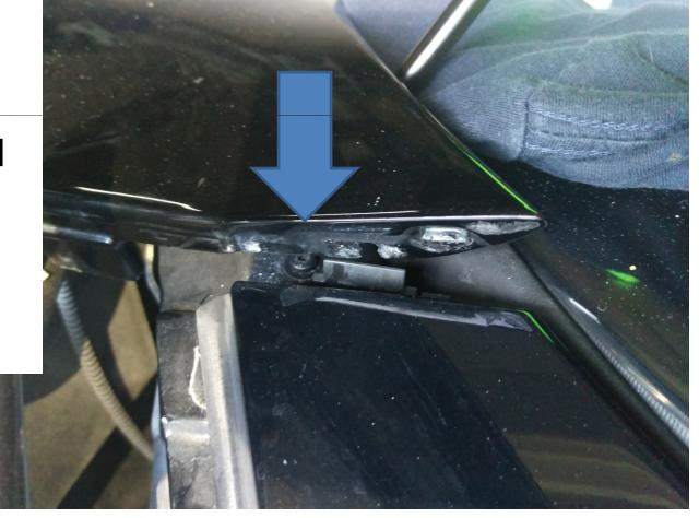
7. From under the car, there are three 10mm nuts that hold the fender to the front bumper. Remove these (A ratchet socket or cordless drill with an extension will help here)
