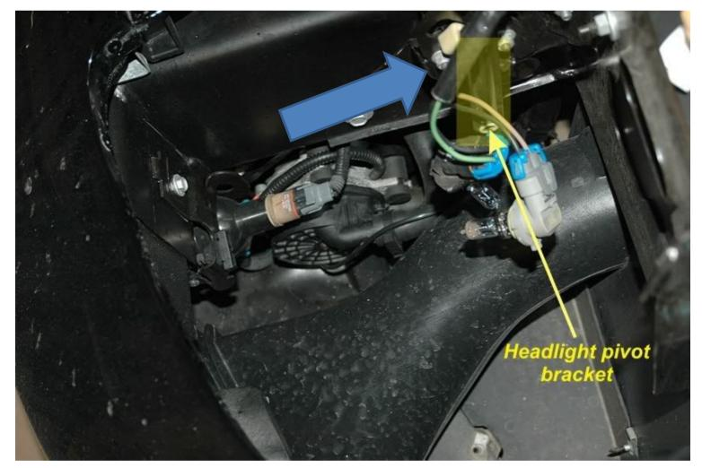
5. There are 5 mounting points that hold the frame in place (shown below) Three 10mm nuts on the wheel well and two 13mm bolts on the frame rail. Make sure to save these as they will be used to mount your new lights. Be Careful not to scratch your paint when removing the frame. (note: the 4"x4" headlight control box shown here bolted to the headlight frame will be removed and the harness connectors taped off. The control box will not be reused with the new lights.
