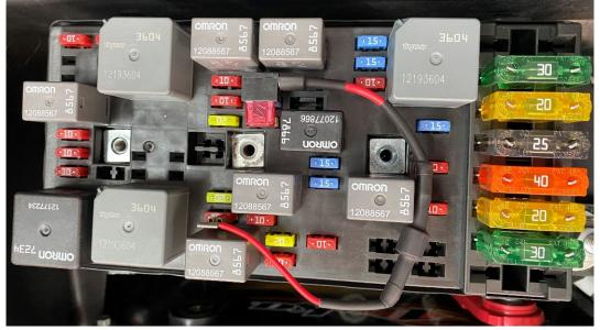
Included Fuse Factory #10 fuse goes in lower slot
