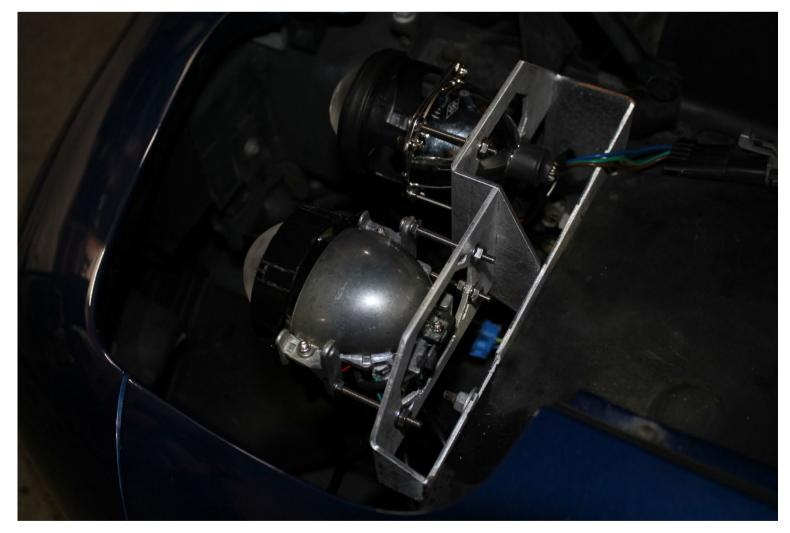
9. Identify your low and high beam connectors and note the position of the black (ground) and colored (12v+) wire
