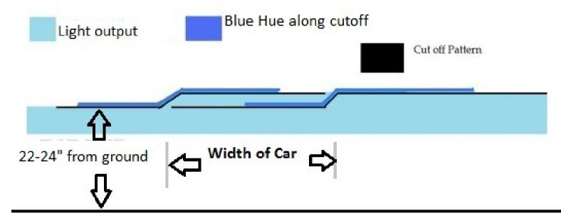
There are 3 types of adjustment: Rotation, Vertical and Horizontal. Vertical and horizontal adjustment are accomplished by loosening the flange nut on one side of the frame and tightening the one on the other side. Rotational ad
