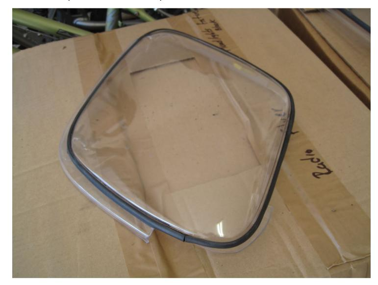
14. Install the "D" profile weather strip around the main lens as shown
