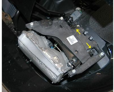
4. With the headlight tilted down, remove the 10mm nut that holds the headlight lifting arm to the headlight motor. Disconnect the headlight bulb sockets and remove the headlight (picture shows the placement of the nut without the headlight.
