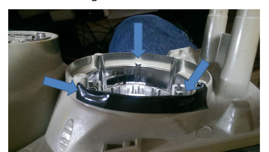
3a. Install a section of electrical tape (about 1.5-2") on the INSIDE of the U shaped weatherstrip as shown with sticky side facing AWAY from the side with cutouts. Then mount the weatherstrip on the lip of the headlight housing with the cutout side facing inward lining up with the bolt mounts as shown
