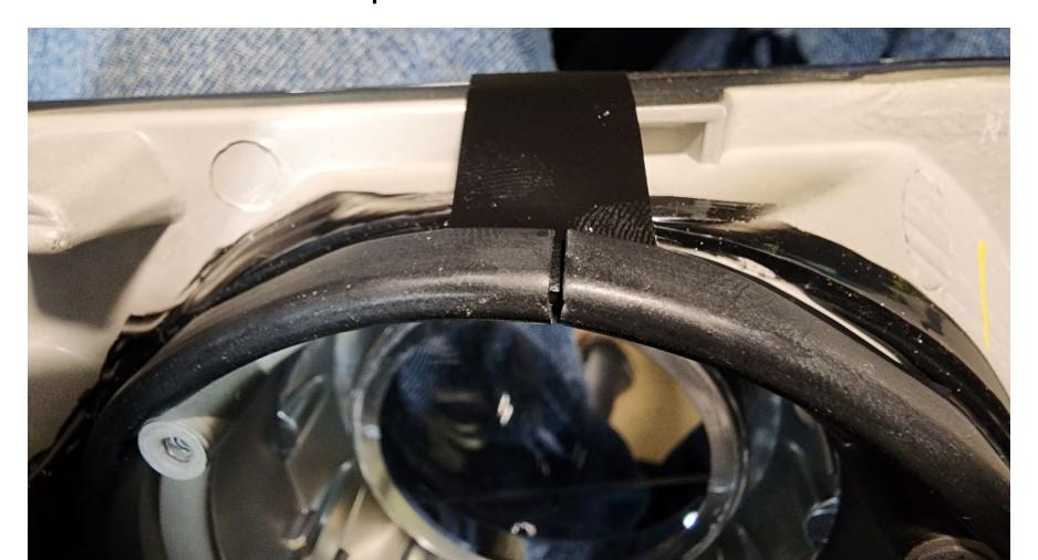
3c. Wrap the electrical tape around the outside of the U-profile weatherstrip and attach it to the inside lip of the headlight housing as shown. (this provides a complete seal with no gaps when compressed by the new projector assembly weather seal.
