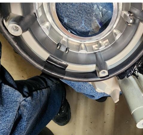
4. The provided spacers have a lip. This lip slips under the foam weatherstrip to help hold it in place during installation. Line the spacer up with the holes in the aluminum plate. (Nova Edition projector show, but this applies to both projectors)
