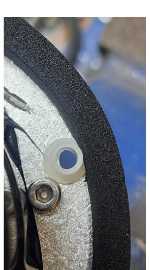
5. Insert the screws provided from the back side of the projector plate through the spacer. The combination of screw and spacer will hold both in place during installation. (Nova Edition projector show, but this applies to both projectors)
