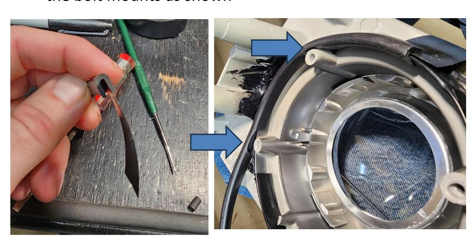
3b. Bring the other end of the U profile weatherstrip around and open it up to allow it to stick to the electrical tape so that both ends of the weatherstrip are mirroring each other with the electrical tap in the middle.
