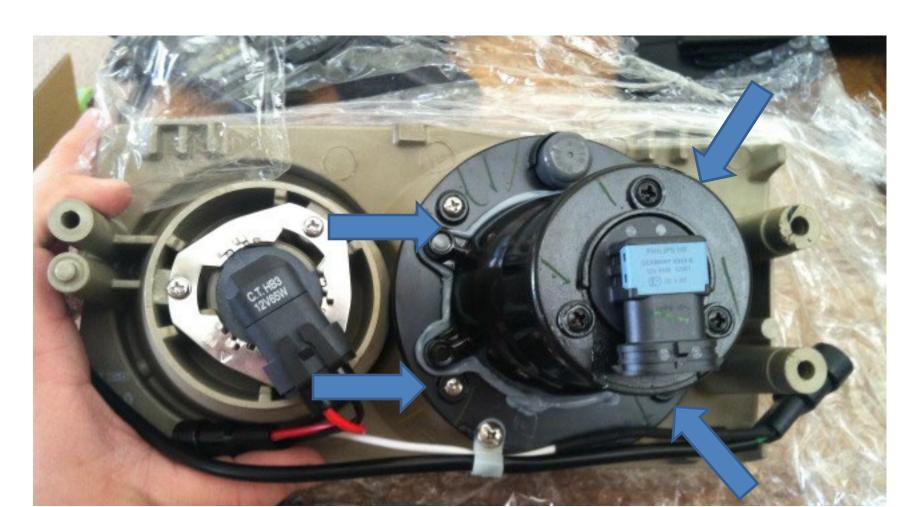
2. Break off the knob marked by the arrorw and use a small strip of electrical tape folded over to block off the cutouts on the bottom part of the housing.
