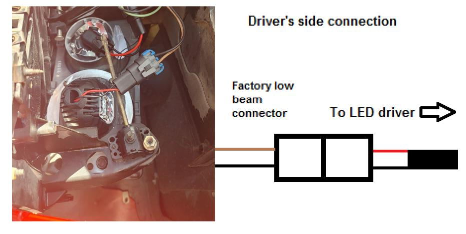
10. On the passenger side, connect the lifting arm to the motor shaft, then connect the small relay harness with male and female headlight connections between the factory low beam connector and projector as shown. Make sure the polarity is correct on the connections (black wires should line up with the black wire on the harness and black wire to the projector
