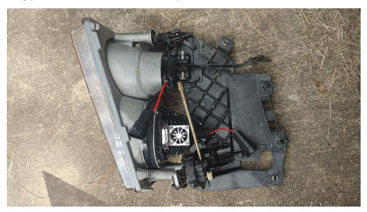
Suggested note: The mounting screws are self-tapping. To help avoid cracking the mounting points from the pressure of the cutting threads, insert the screw one turn then back the screw out and clear the debris. Tighten two turns, then back out and clear debris. Continue until the mounting hole is fully threaded.
