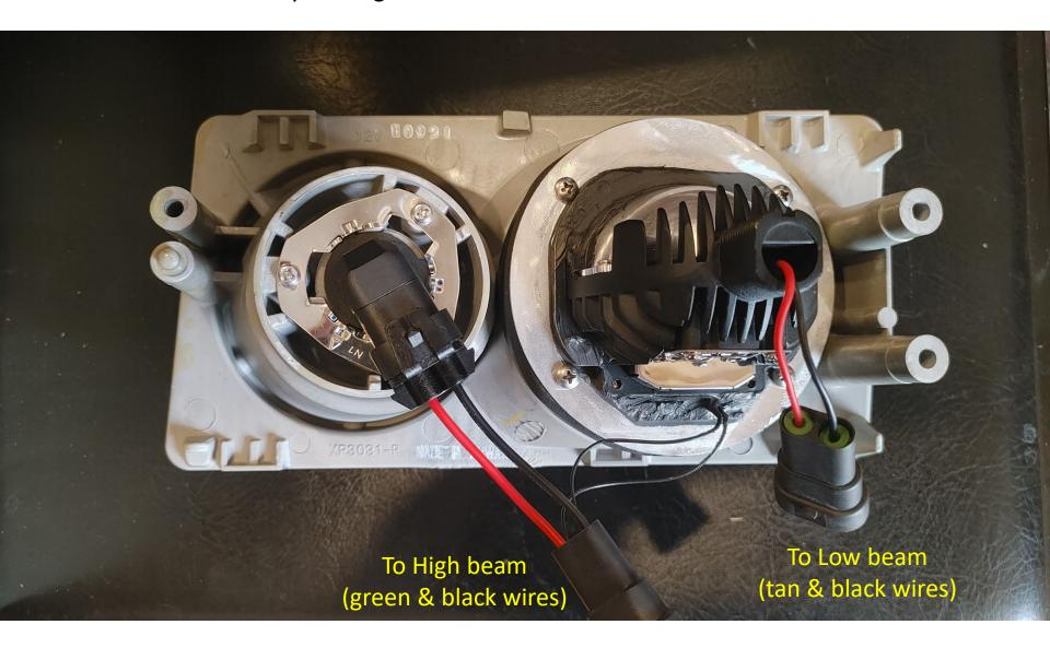
9. Set the headlight in the opening and secure the lifting arm to the headlight motor shaft. On the driver's side connect the factory low beam connector (tan and black wires) directly to the LED wires coming out of the back of the projector. Then connect the high beam (green and black wires) to the connector that goes between the high beam bulb and wires coming from the bottom of the projector.
