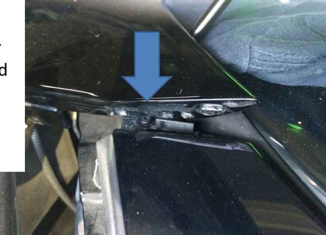
7. From under the car, there are three 10mm nuts that hold the fender to the front bumper. Remove these (A ratchet socket or cordless drill with an extension will help here)
