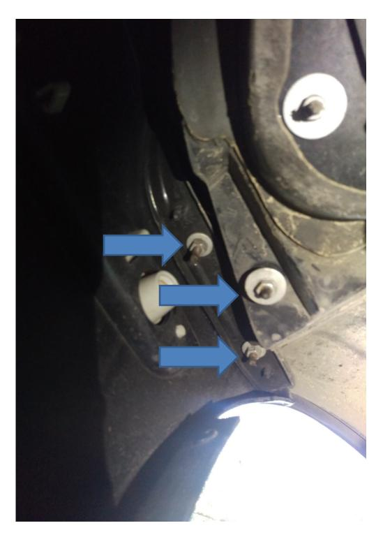
Three 10mm nuts with large washers hold the headlight in place. Remove these nuts to release the headlight.
