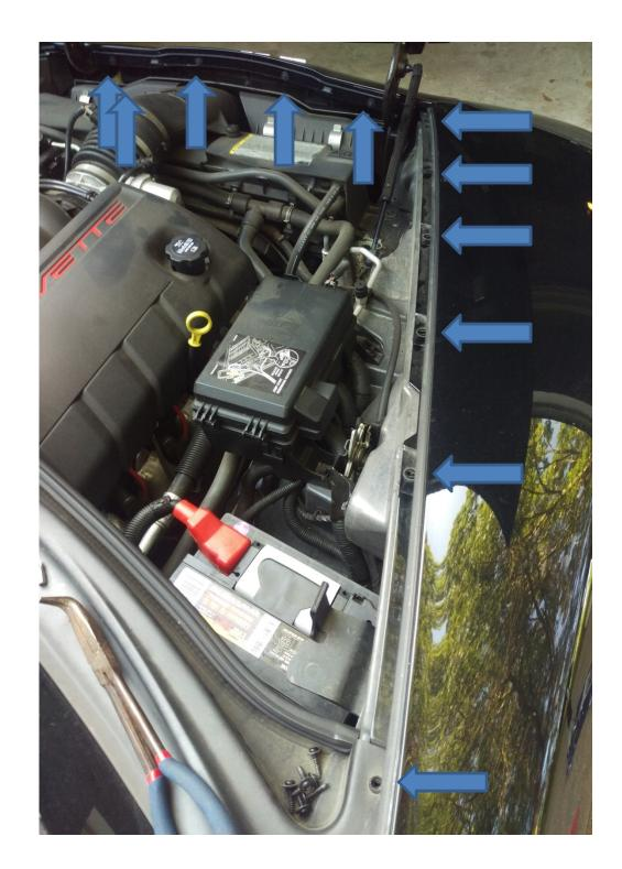
Firmly lift the front bumper to reveal an additional Torx 15 screw on the fender. Remove this screw.
