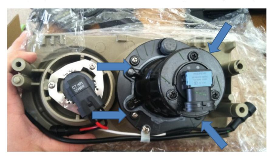
2. Break off the knob marked by the arrorw and use a small strip of electrical (or other type of waterproof tape) folded over to block off the cutouts on the bottom part of the housing.
