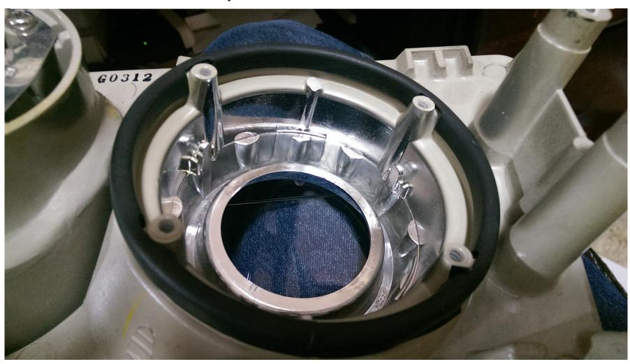
4. Insert the factory projector mounting screws into the mounting holes of the new projector assembly. Insert the provided spacers on the end of the screws as shown.
