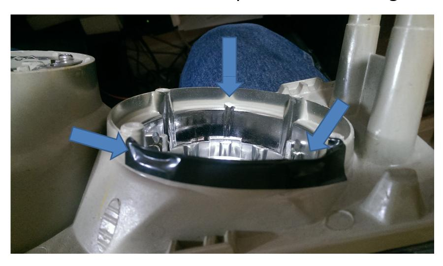
3. Install the pre-cut weather seal around the circular edge of the housing (lining up the cutouts in the weather seal with the boltholes as shown)
