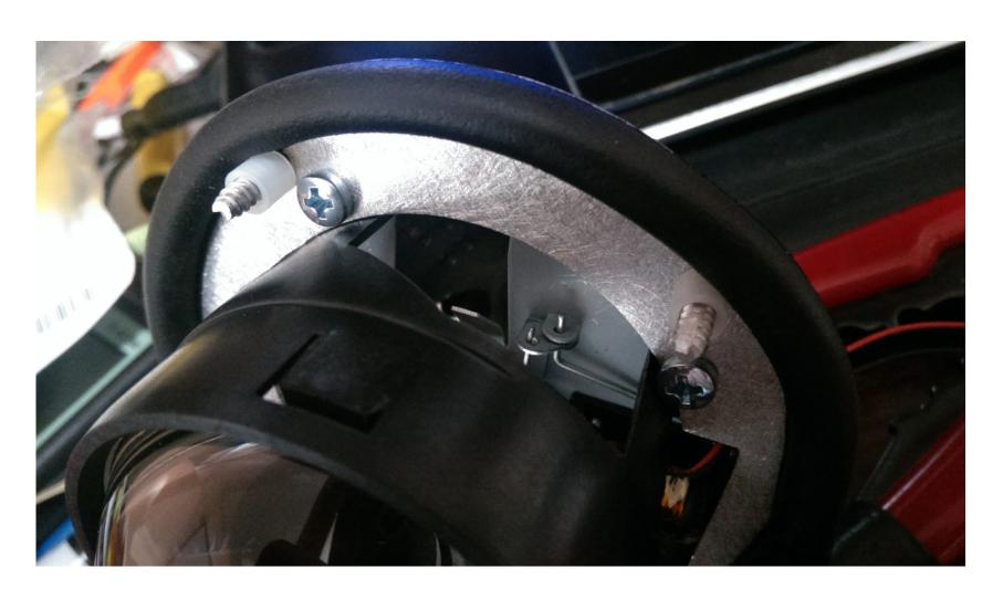
5. Install the new projector on the factory housing making sure the spacers remain on the screws and the bottom of the projector has wires coming out of the seal. Hand-tighten the screws gently.
