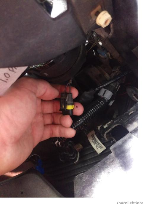
This is what the connector looks like with the pin lock removed. Note the position of the black and purple wires. Purple is the positive wire black is the ground. These will need to be reversed.
