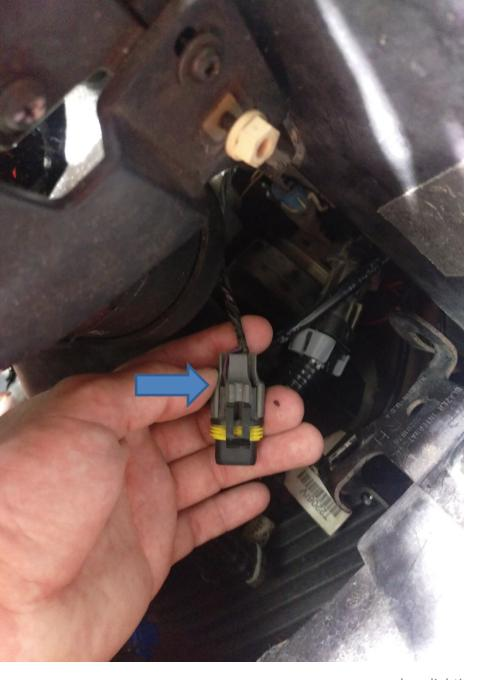
Identify the fog light connector and remove the gray pin lock.
