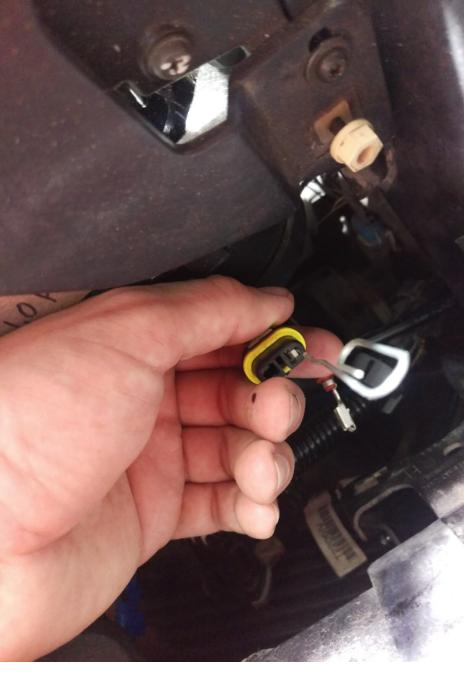
Insert the end of the paper clip into the position shown on the fog light connector. this releases the lock on the pin allowing the pin to be removed.
